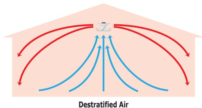
J&D's JD360 Destratifier fan creates low-air-speed vertical air movement providing a comfortable and uniform environment.
